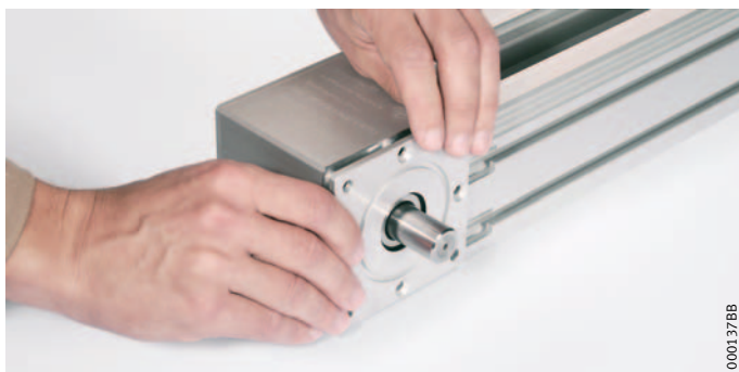
Figure 12 Removing the bearing cover
