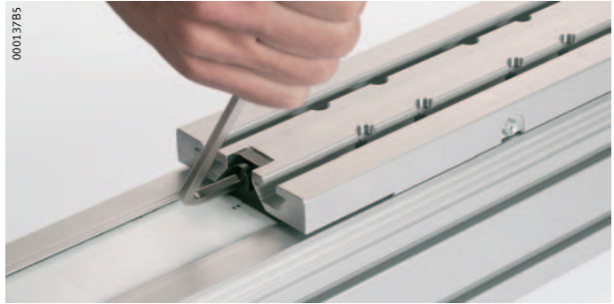
Figure 27 Screw mounting the clamping device to the carriage
