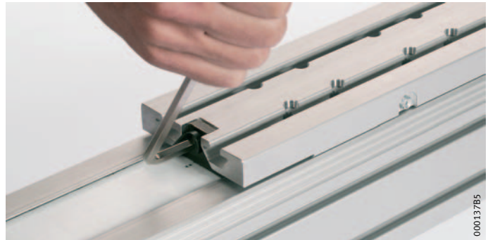
Figure 8 Loosening the adjusting screw
