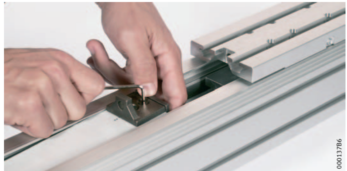
Figure 9 Loosening the fixing screw
