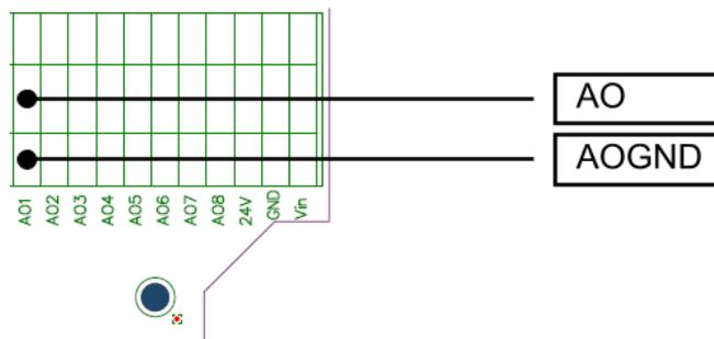
Connecting an analog output (using AO1 as an example)
