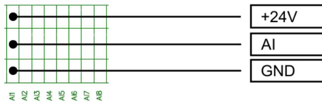
Addition of an analog signal (with AI1 as an example)
