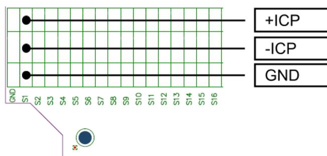
Sensor connection (using ICP sensor 1 as an example)
