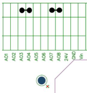
Analog outputs, bridges for the internal power supply
