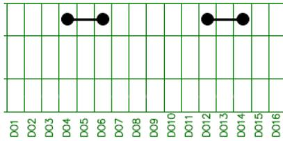
Digital outputs, internal power supply, D1GND/D2GND connected to GND
