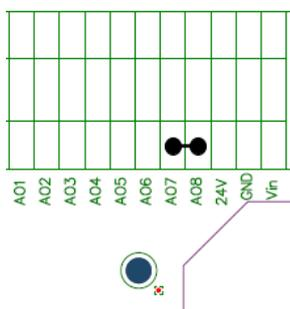
Analog outputs, internal power supply, GND connected to AOGND
