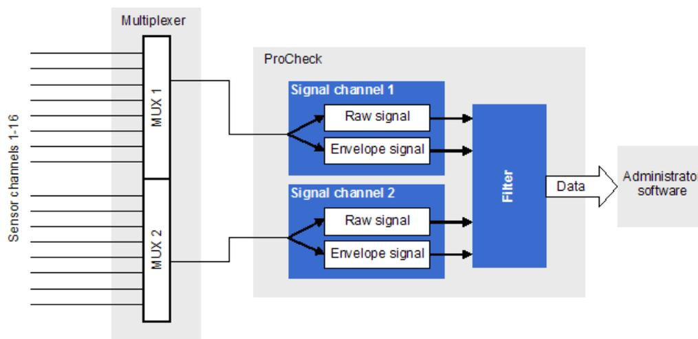
ProCheck signal processing with multiplexer
