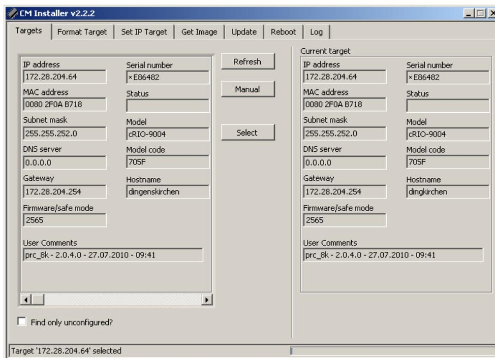
The CM Installer looks for ProCheck devices on the local network by means of a UDP broadcast. If there is a router between a ProCheck device and your computer, the CM Installer usually cannot find the device as the router does not forward the broadcast. In this case, you must enter the IP address of the device manually:
