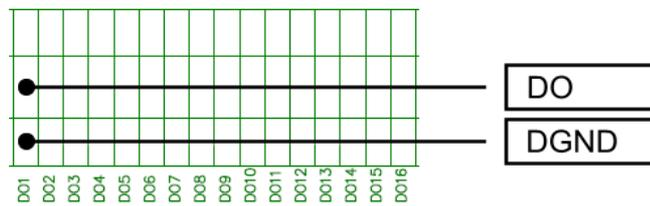
Connecting a digital output (using DO1 as an example)
