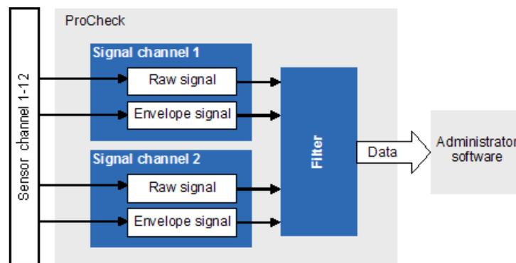
ProCheck signal processing without multiplexer
