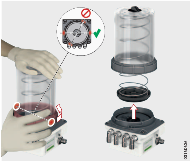
Figure 5 Detach the upper housing part
