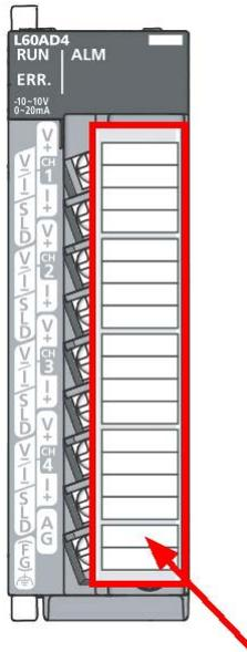
The terminal block cover serves to prevent contact, which would otherwise cause an electric shock. You can mark the adhesive label on the cover to designate the individual terminal clamps.
