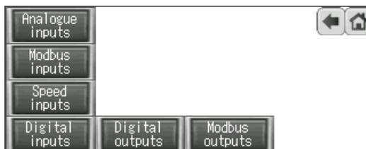
On this page, you can directly display the contents of the FAG SmartController registers for each individual input and output. In particular, this option makes it easier to commission the device. Details on the different options can be found in the following sections.
