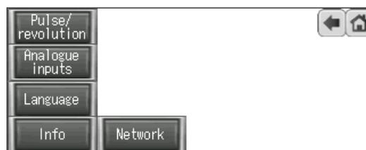
The buttons allow you to access the individual settings options, such as setting the pulses/revolution for calculating the rotational speed or setting the operating mode for the analogue inputs. Details on the settings options can be found in the following sections.
