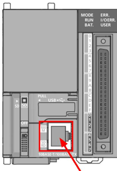
As soon as the FAG SmartController is connected to the network, you can establish a connection to a maximum of 25 FAG SmartCheck devices [\[43\]](#). For this purpose, the network parameters of the FAG SmartController have the following factory default settings:
