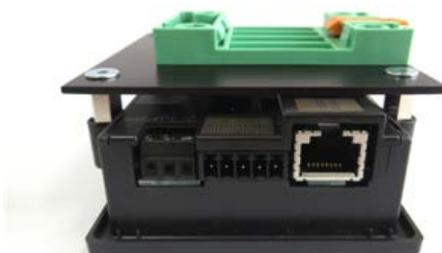
2. Hang the display on the DIN rail using the securing mechanism and lock the tabs. Details on this step can be found in the section entitled **Mounting the FAG SmartController on a DIN rail** <sup>[14]</sup>.
