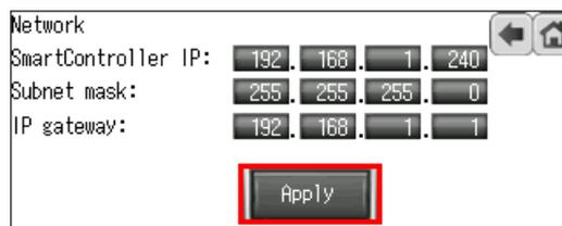
2. Press **Apply** to confirm the changes. Use the navigation elements in the upper right-hand corner to return to the main screen.
