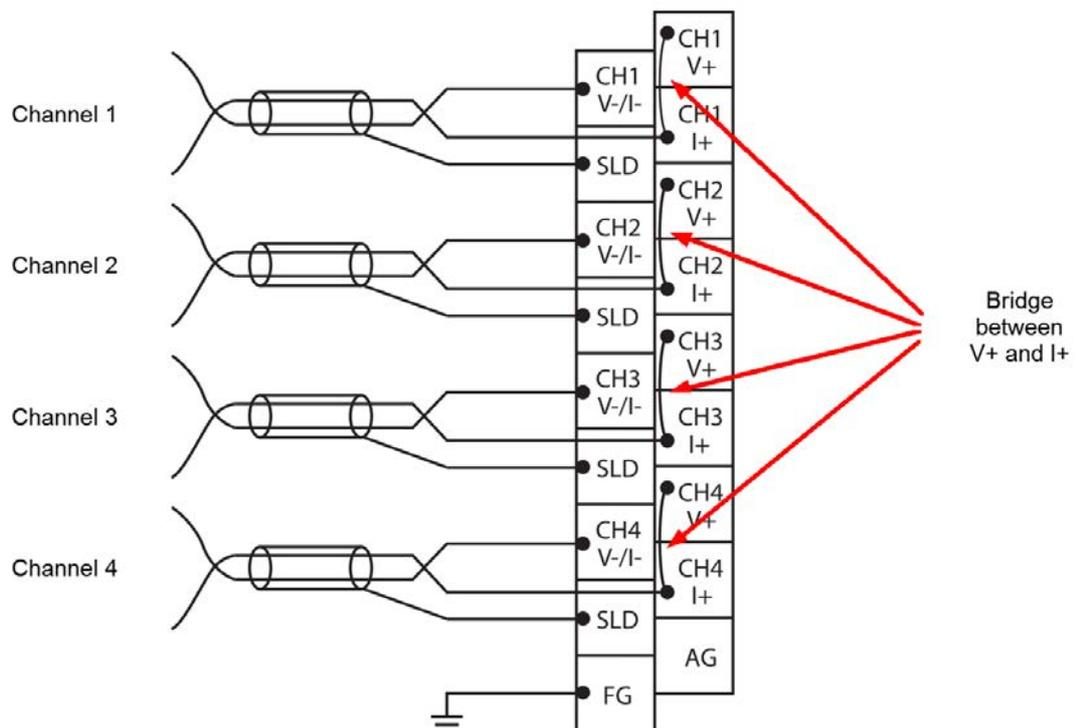
The following illustration, showing the circuit of the analogue inputs, highlights why a bridge between V+ and I+ is necessary with current inputs:
