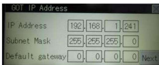
5. Close the **GOT IP Address** window by pressing the **X** in the top right-hand corner and confirm the security prompt by pressing **YES**:
