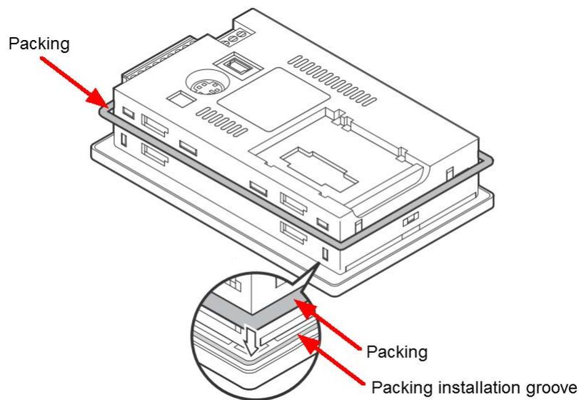
3. Insert the touchscreen display into the panel cut-out from the front:
