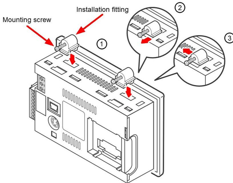
5. Tighten the four screws of the installation fittings to a torque of 0.20 Nm to 0.25 Nm.
