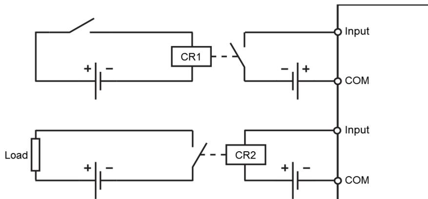
**Connection of external peripherals to the inputs and outputs**
