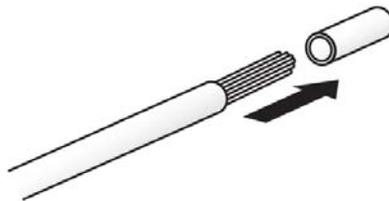
2. Push a ferrule onto the stripped end of the wire and firmly press it in place.
