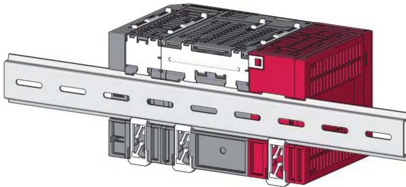
4. Place the securing clips on the DIN rail and secure them.
