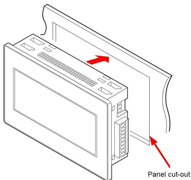
4. Assemble the supplied installation fittings. The following installation diagram shows how installation fittings are inserted into the openings provided for this purpose **(1)**. To secure the fittings in position, first slide each fitting to the rear of the display **(2)** and then to the left **(3)**:
