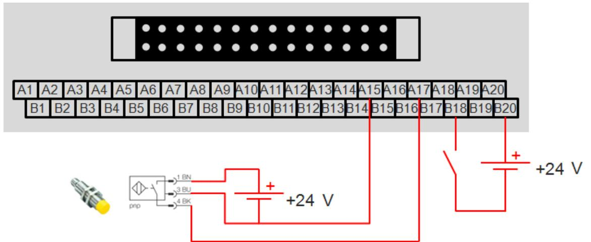
The circuit diagram for the digital logic inputs is as follows:
