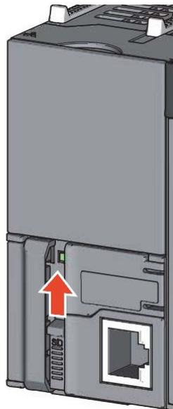
2. Open the cover of the slot and press the SD card to release it. Then remove the card.
