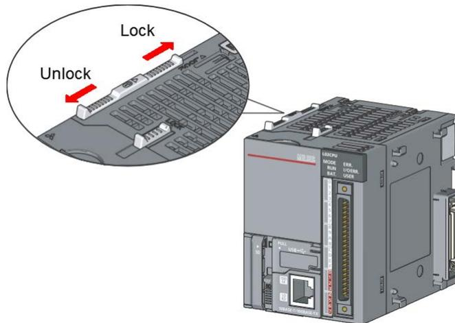
Accordingly, you have to slide the connecting latches in the opposite direction if you want to connect the modules together again.
