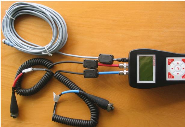
*Ferrites attached to sensor cables*
