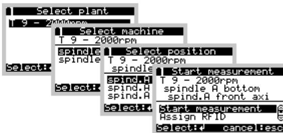
*Starting the measurement after selecting a measuring point*
