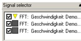
Click the preferred signal. The signal you have chosen is highlighted by the cursor signal (yellow triangle). As soon as you have positioned the basis cursor on a diagram value, the corresponding values are connected in the other diagrams by a transparent yellow plane.
