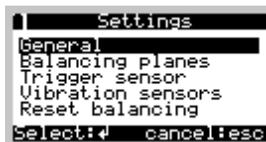
You can also restart the balancing measurement (menu item **Restart balancing**). This resets all balancing measurement data.
