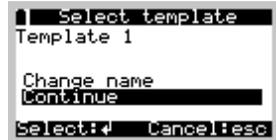
In the next menu you can change the template name so that the free measurement can later be assigned to the measuring point at which it was recorded.
