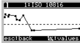
In the trend view you can use the cursor key ▲ or ▼ to switch between the several trends. A horizontal line in the diagram indicates the main alarm limit. A horizontal broken line indicates the pre-alarm limit. In the middle of the window number and type of the characteristic value are displayed. Individual measurement points (■) are joined by lines.
