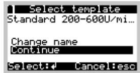
In the next menu you can change the template name so that the free measurement can later be assigned to the measuring point at which it was recorded.
