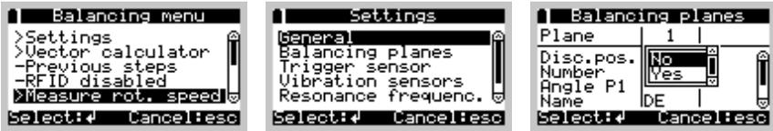
When carrying out a free measurement all other values can be changed in addition to the template name. To do this, select the **Settings** item in the menu. You can now select the relevant values using the Enter button  $\leftarrow$ . Depending on the type of setting, you can now type in a new value directly, make a selection from a drop-down menu or modify an item of text as described above. Leave the settings menu with the Esc button  $\leftarrow$ .
