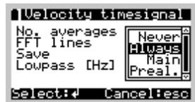
When carrying out a free measurement all other values can be changed in addition to the template name. To do this, select the **Settings** item in the menu. You can now select the relevant values using the Enter button **↵**. Depending on the type of setting, you can now type in a new value directly, make a selection from a drop-down menu or modify an item of text as described above. Leave the settings menu with the Esc button **esc**.
