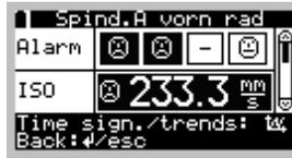
In the "Alarm" line, an alarm status overview of all characteristic values is displayed. A scrollbar is displayed on the right of the display if more than one characteristic value exists. Characteristic values with exceeded main alarm limits are highlighted.
