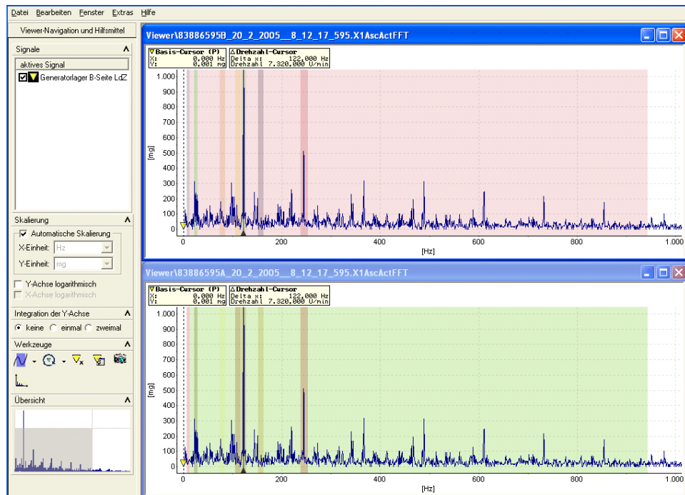
Fault analysis case study using imbalance as an example
