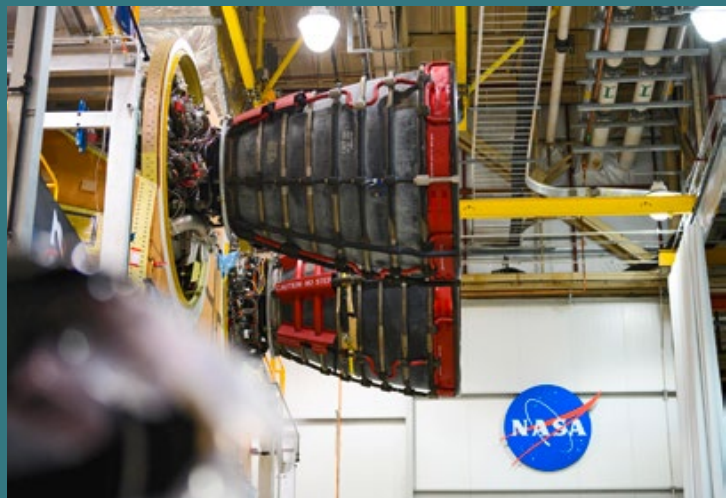
Rocket engines with Schaeffler bearings in the turbo pumps
