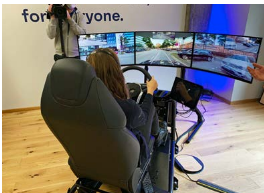
360-degree view on three monitors: The teledrivers from car-rental service Vay watch traffic as shown here during a test run
