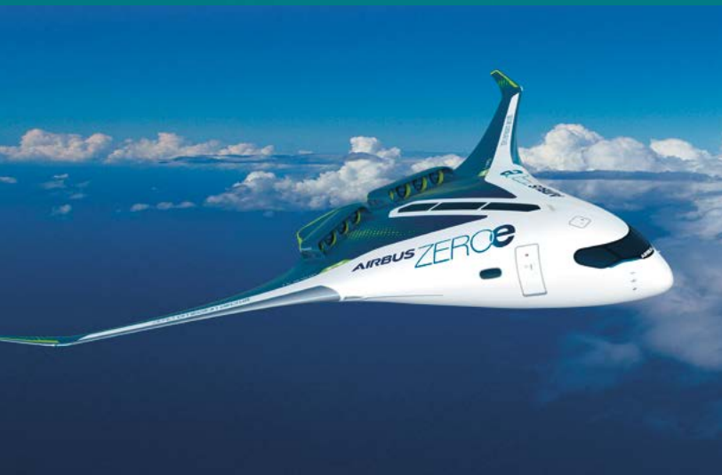
ZEROe is an Airbus concept aircraft. Two hybrid hydrogen turbofan engines provide thrust for the blended-wing-body aircraft. The liquid hydrogen storage tanks are installed underneath the wings
