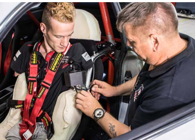
A seat adapted to his specific needs provides Janis McDavid with the required support in the BMW M3. He uses the joystick in his left armpit to drive the high-tech race car
