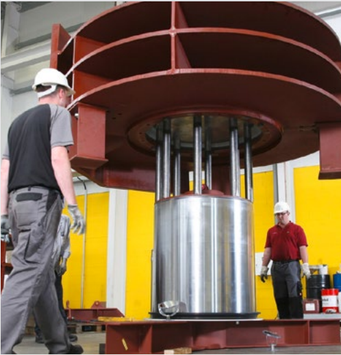
Installation of a large housing with assembled spherical plain bearing for an offshore platform
