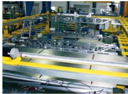
Inside the transformer sheet handling and positioning system from Tuboly-Astronic, AG, including a total of nine INA linear and tandem actuators
