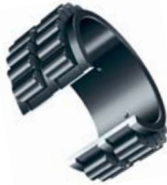
Cylindrical roller bearing with Durotect® B coating: Lower wear and friction levels, for example in wind turbine gearboxes
