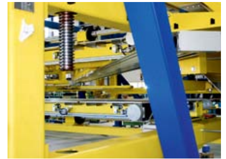
Swivel arm drive and guidance system for yoke sheet I for rotating and positioning the yoke sheets by 90° from the longitudinal to the transverse direction using an MDKUSE-25 tandem actuator from INA
