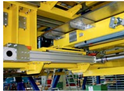
Transverse adjustment unit of the linear transport system for eccentric yoke sheets with one of two MKUSE-25 linear actuators from INA
