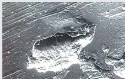
Microspalling (SEM image)
