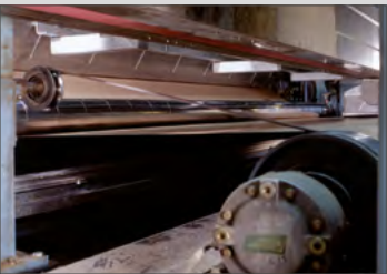
Spreader rolls allow crease-free guiding of material webs
