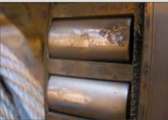
Damage to rolling element of tapered roller bearing
