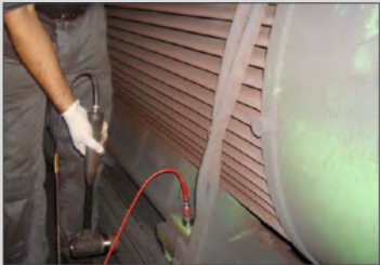
Sensor positions at support of the motor for bump test
