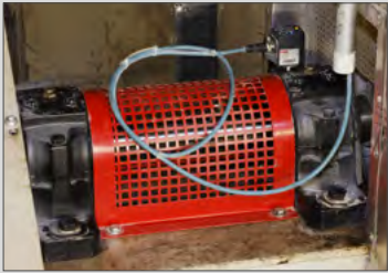
Ventilation unit: The FAG SmartCheck is fitted to the shaft's bearing support
