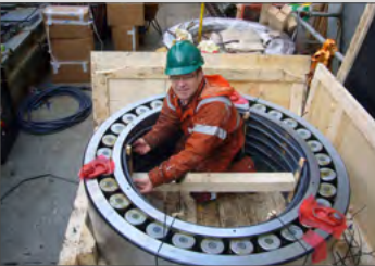
The flexible inductors are wound around the bearing
