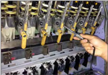
Manual vibration check on texturing units with friction unit spindles
