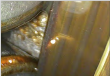
Damage to the raceway of the inner ring
