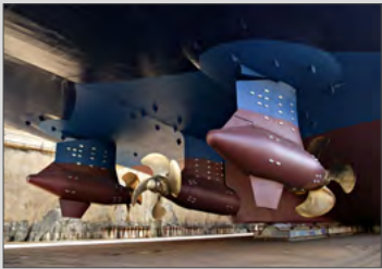
Energy-efficient Azipod® propulsion systems from ABB are proven and established in cruise ships
