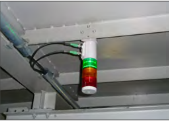
Simple visualization of the operating condition with the help of the FAG SmartLamp
