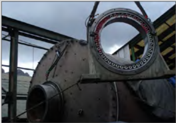
For mounting of large size bearings expert knowledge and expert tools are required
