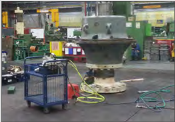
Mounting work on site – here: shaft and housing unit
