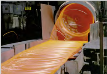
The still red-hot wire is brought into shape
