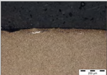
“White etching cracks” (WEC) underneath the raceway material
