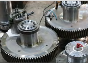
The heaviest gear weighs almost five tons and has an outside diameter of 1 700 mm
