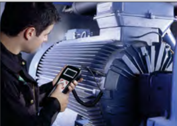
FAG Detector III can monitor pumps and compressors amongst others
