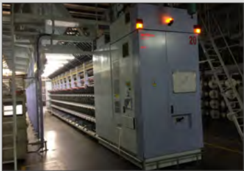
Barmag texturing machine with INA-brand friction spindles
