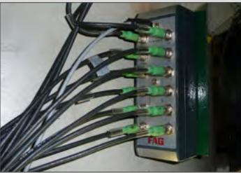
The FAG SmartConnect Box allows the power supply and additional signals to be distributed
