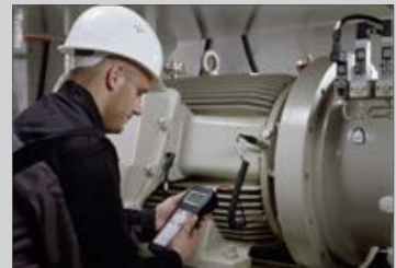
Dispositivo de Condition Monitoring offline FAG Detector III
