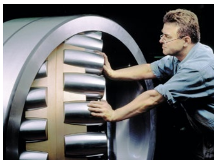
Reconditioning of large size bearings
