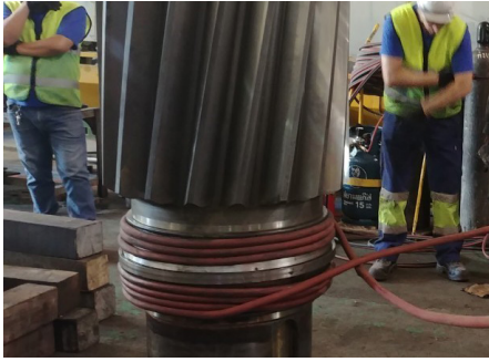
Bearing dismounting by heating leftover bearing inner ring on the shaft
