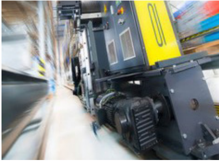
One of the seven automated storage and retrieval systems that are monitored using SmartChecks in the EDC Central in Kitzingen (drive)
