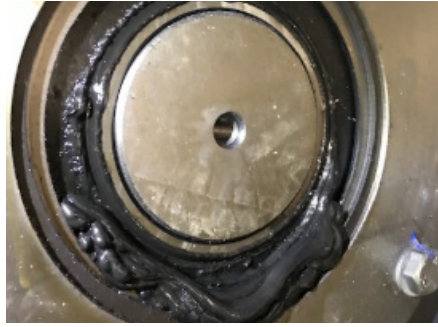
Grease has escaped from a bearing in the drive of a storage and retrieval system
