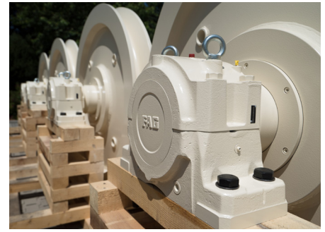
Close-up view of rope sheaves with FAG plummer block housings and internal spherical roller bearing
