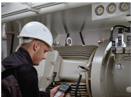
Dispositivo de Condition Monitoring offline FAG Detector III
