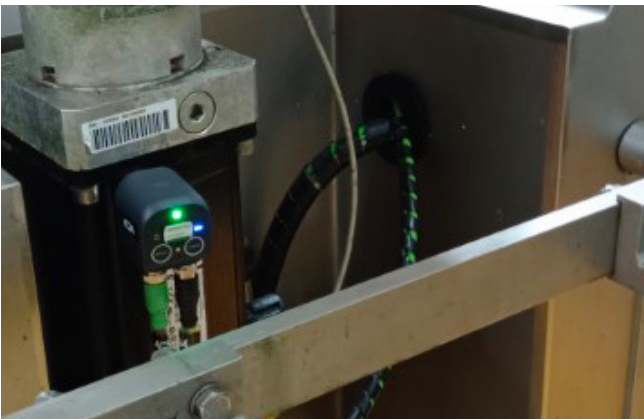
SmartCheck installed on servo motor.
