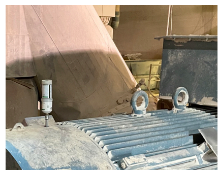
Pilot: OPTIME C1 lubricator is mounted on a motor
