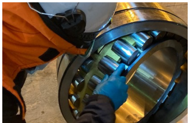
Employee checks the bearing clearance.
