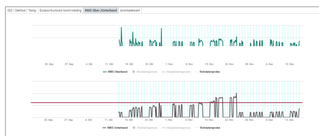
Figure 1– Fresh air fan product cooling oven 1: low frequency vibration increased, which indicated an imbalance in the fan.
