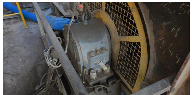
OPTIME CM sensors on a non-driven side of the fan
