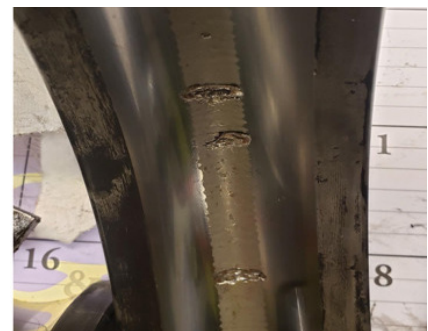
OPTIME has identified bearing damage.
