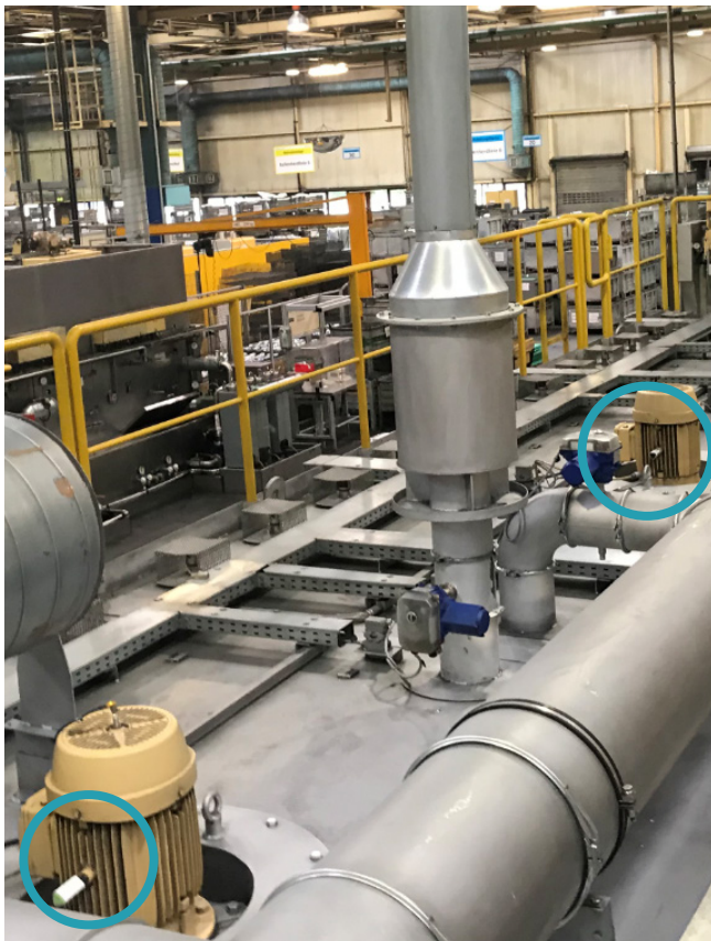
OPTIME sensors on motors
