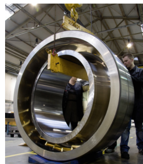
Ready to install: huge spherical roller bearings with a brass cage, an outer diameter of 1,420 mm, and weight of over three tonnes.
