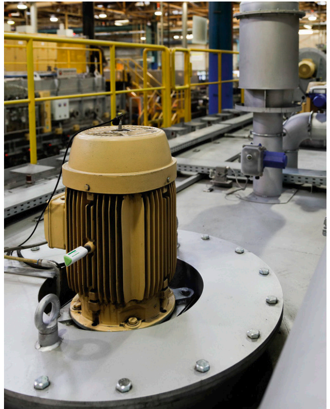
Rapidly installed: A machine monitored with OPTIME in the hardening at Schaeffler in Schweinfurt
