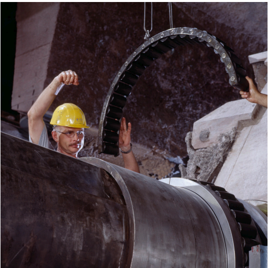
Simplified bearing replacement, thanks to a split spherical roller bearing
