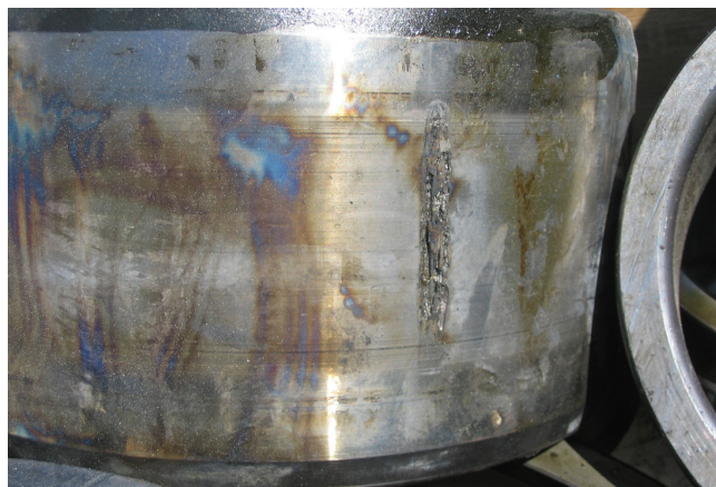
Detected bearing damage
