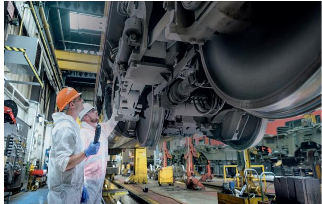
Digital maintenance: The DMC on the axlebox bearings allows SBB to correlate damage patterns with operating data like service life, route profile or wagon load.
