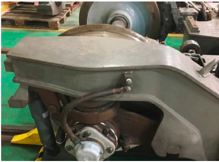
The CM test rig can accommodate complete railway wheelsets
