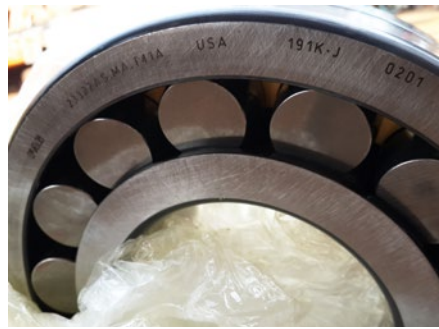
FAG spherical roller bearing for vibrating screens
