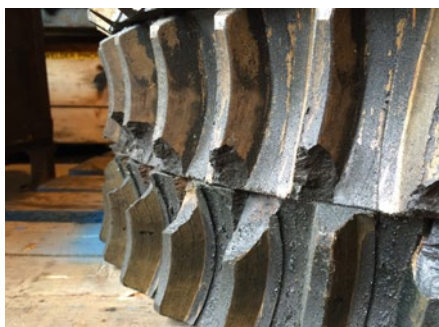
Damaged brass gear
