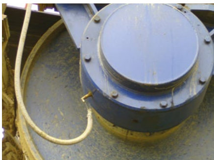
Lubricant connection to the belt conveyor drum bearing
