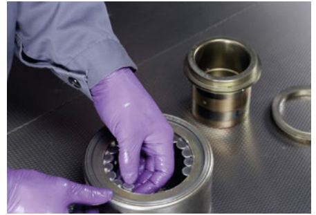
Greasing of the bearings
