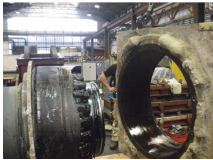
Dismounted spherical roller bearing with outer ring damage
