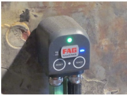
Monitoring of grinding roller bearings using the FAG SmartCheck
