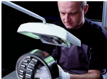
Checking and assessing bearings
