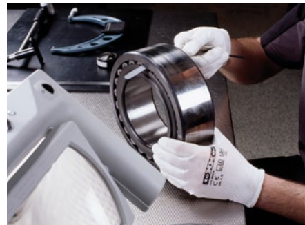
Checking of bearing clearance
