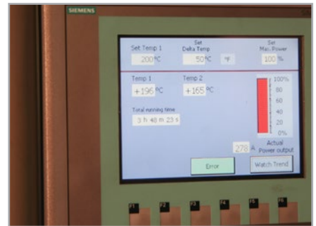
The heating process is controlled using a touchscreen display on the FAG Heater5000
