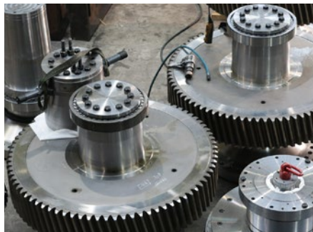
The heaviest gear weighs almost five tons and has an outside diameter of 1 700 mm
