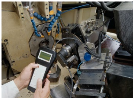
The FAG Detector III is a handy, easy-to-use offline vibration measuring device
