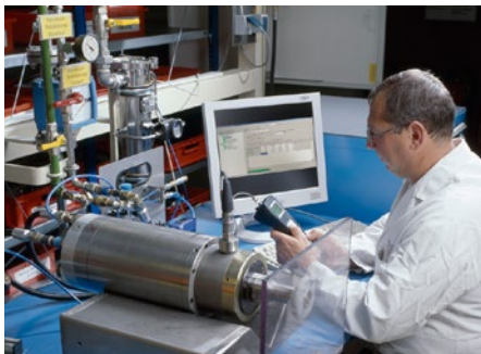
Manual measurement on a spindle test stand
