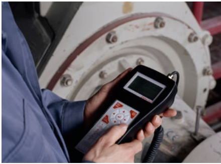
Measuring device for offline vibration monitoring FAG Detektor III
