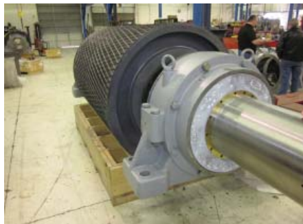
Complete head pulley assembly prior to being belivered to mine site
