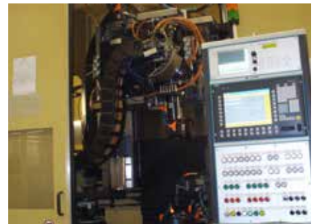
Monitoring of main spindles by FAG DTECT X1 s
