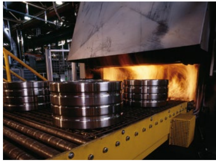
Roller hearth furnace at Schaeffler in Schweinfurt
