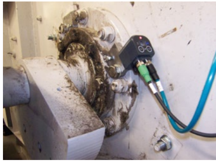
FAG SmartCheck in use on a vibrating screen
