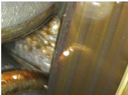
Damage to the raceway of the inner ring
