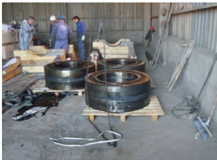
Dismounting of bearings from roller press
