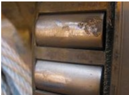
Damage to rolling element of tapered roller bearing
