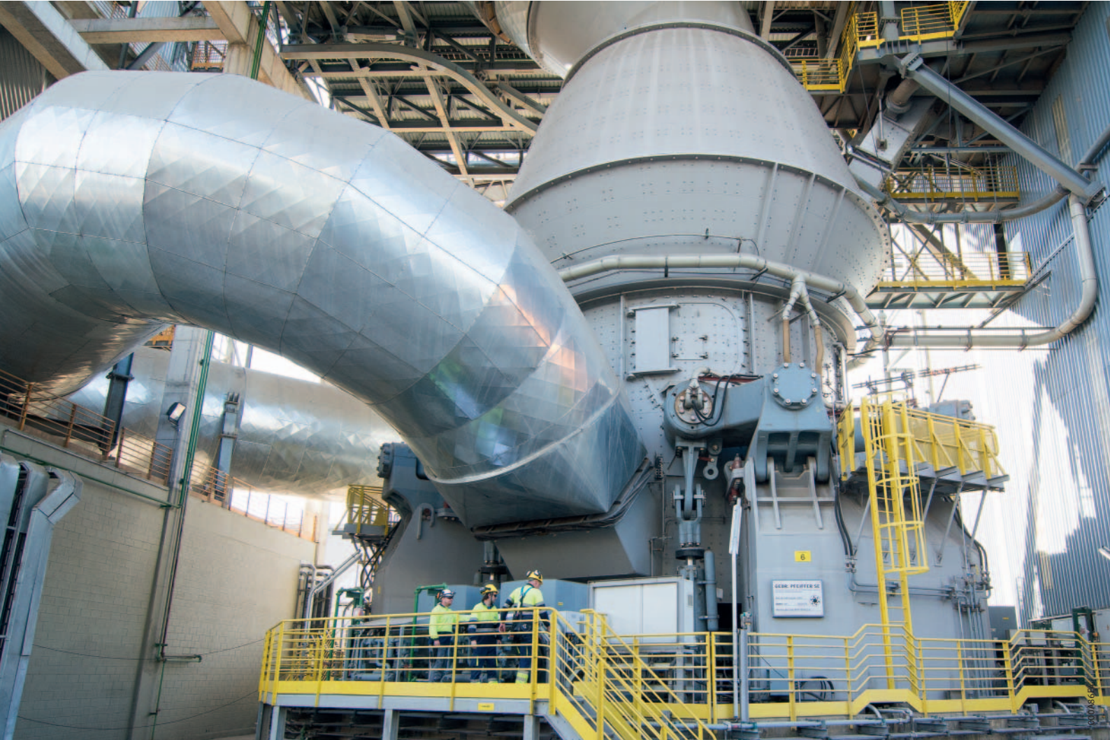
MVR 6700 C-6: The largest vertical mill in the world, producing in Barroso, Brazil
