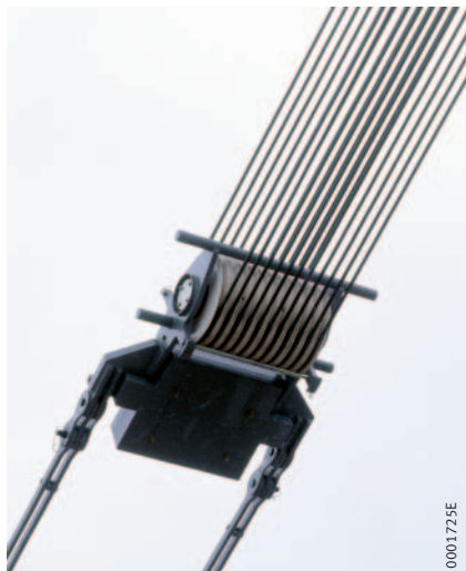
Figure 2 · Cable sheave bearing in the example of an S boom adjustment mechanism between the boom and the derrick arm
